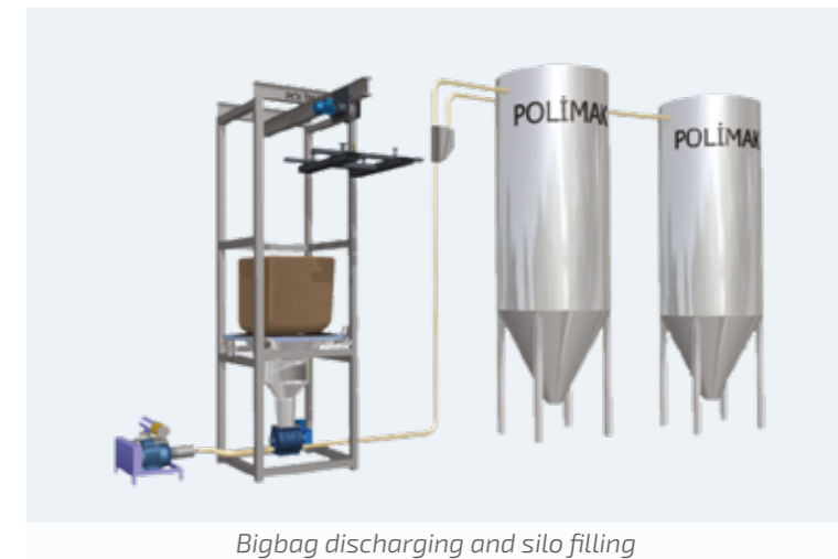
Bigbag discharge, storage, weighing, dosing and conveying system
