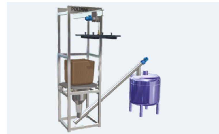
Filling the reactor tank from Bigbag
