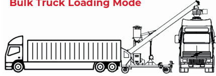
Container Discharge & Bulk Truck Loading
